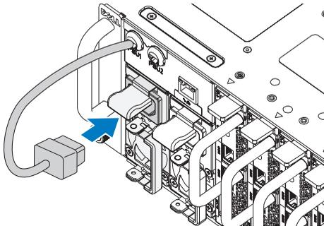
**NOTE:** The correct configuration of the integral chassis AC power cables to the PSU sockets is as shown in the following illustration.
